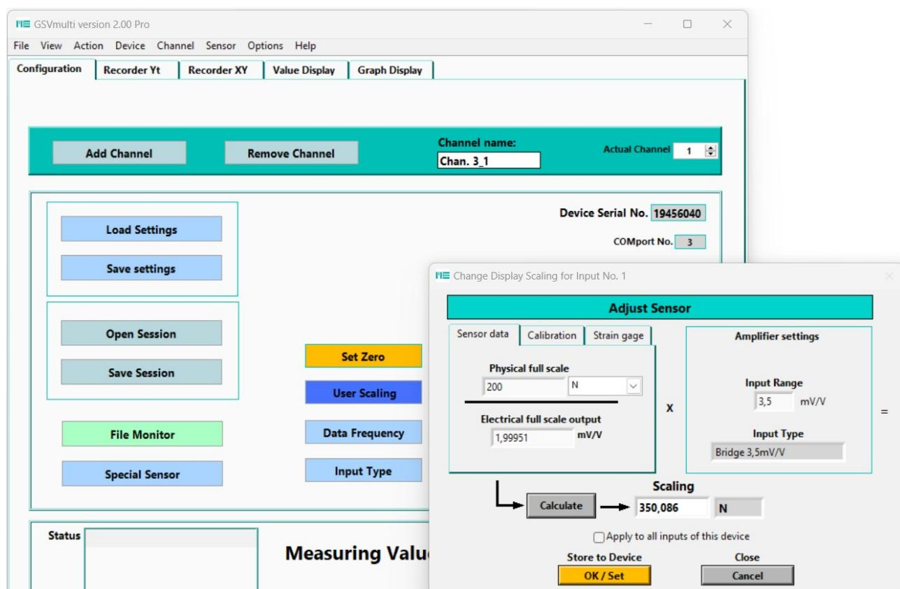
Press Calculate and then **OK / Set**, to save the scaling in the measuring amplifier.
