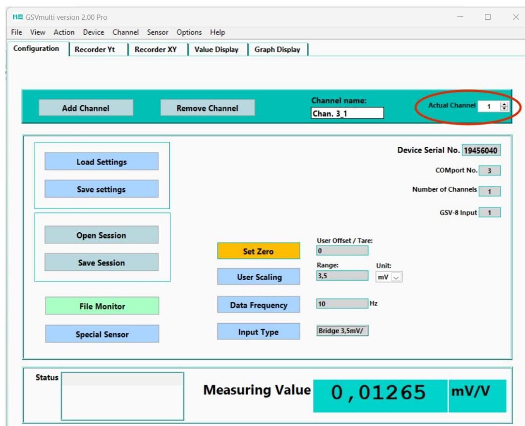
With **Load Settings**, factory settings (default) of the measuring amplifier can be restored and also those that have previously been saved by the user with Save Settings.
