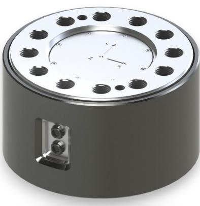
The multi-component sensor K6D300 is suitable for the simultaneous force and torque measurement in three mutually perpendicular axes.
