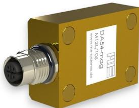
The strain sensors DA54-mag, DA54-tiewrap are suitable for high-resolution detection of forces and deformation of structural works such as bridges, silo legs, offshore wind farms, railway lines, etc.
